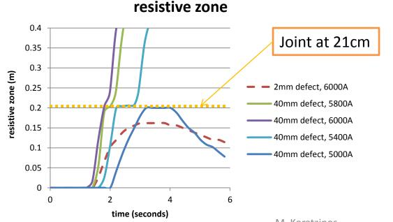
When no propagation is seen to a good joint, there is propagation to a bad joint, even at current levels 1000A less
