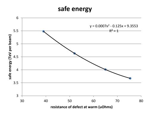
For RB Magnet quenches (propagation through the bus bar) and EE time constant of 68sec
