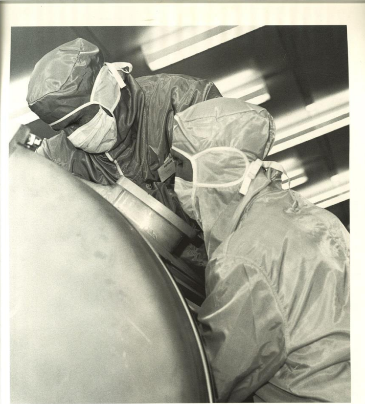
Karl Schirm and Albert Insmoby 'operate' on a superconducting radio frequency cavity in a clean room.
