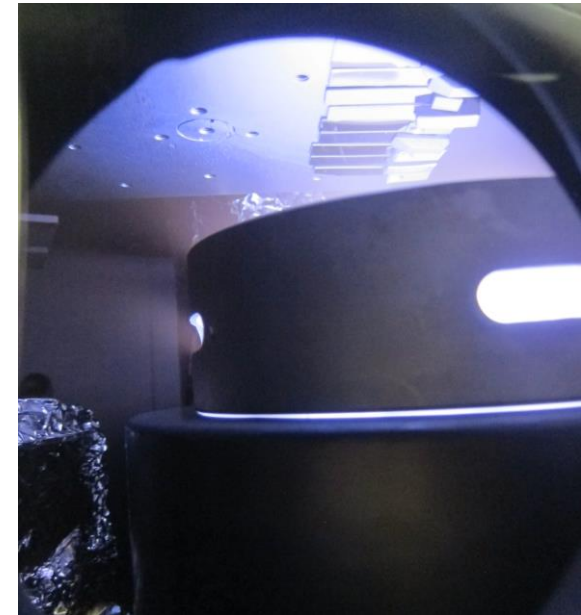
Planar magnetron Nb 3 Sn target sputtering
