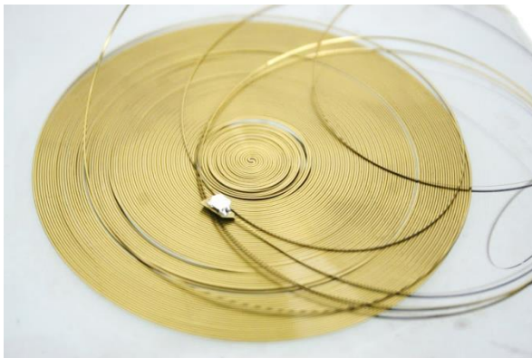
Long flex cable with laser cut. Length over 15meters
