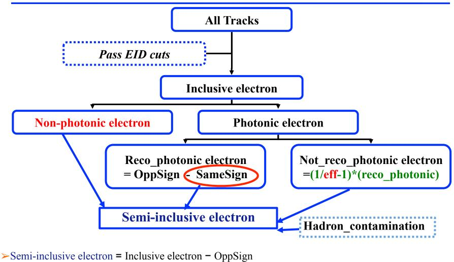
Signal: NPE= Semi-inclusive +SameSign-(1/eff-1)\*reco-photonic-Hadron\_contamination
