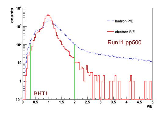
> P is the momentum measured by TPC, E is the sum of the associated BEMC points' energy measured by BEMC.
