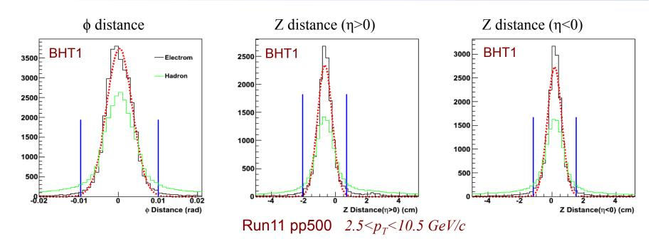
>Projection distance: distance between the TPC track projection position on BSMD  $\eta$  and  $\phi$  planes and the reconstructed BEMC point position
