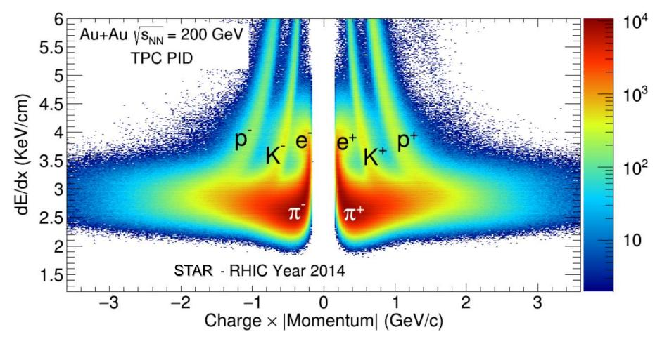
TPC PID: Using energy loss (dE/dx)
