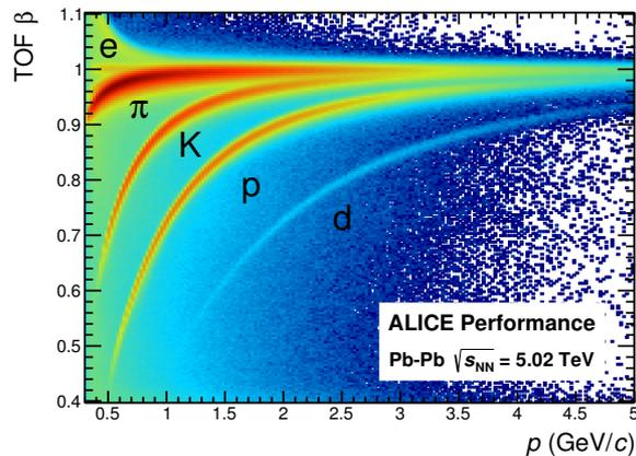
TOF: PID through particle time of flight
