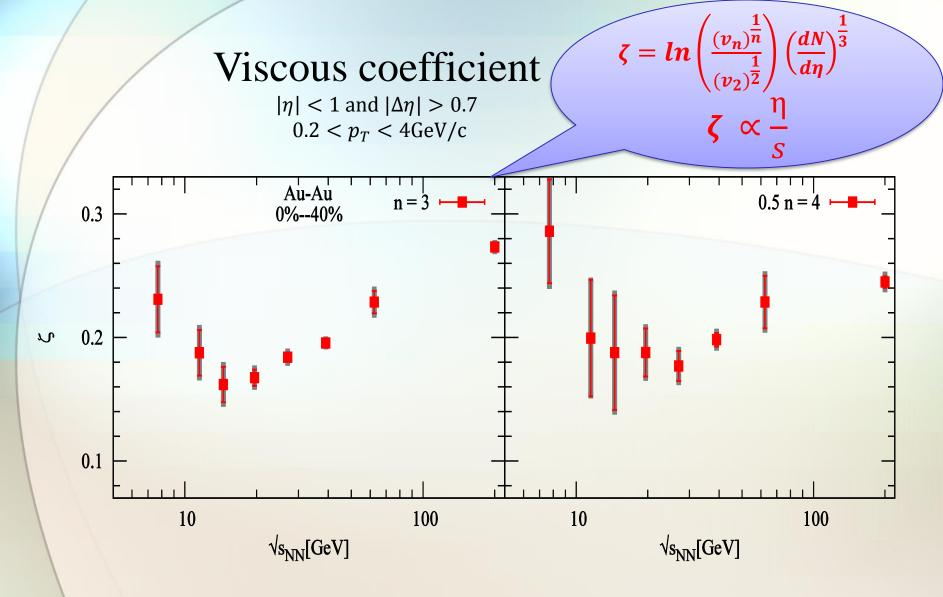
The viscous coefficient  $\xi$  shows a non-monotonic behavior with beam energy in both cases, n = 3 and n = 4.
