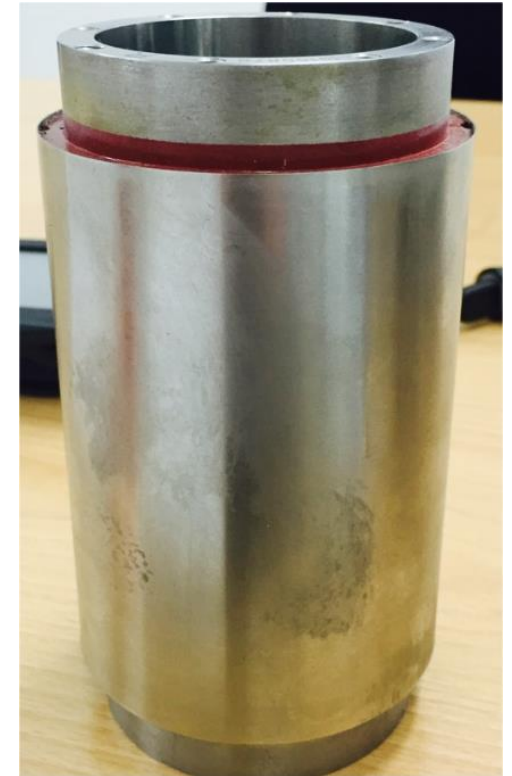
Rotor banding (done by Alxion)
