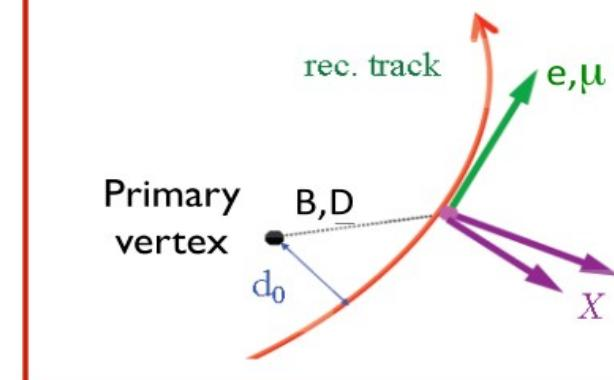
need good PID (in particular e, mu, also K) and vertexing capabilities (sub 100 μm)
