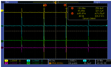
signals from BPM pickup
