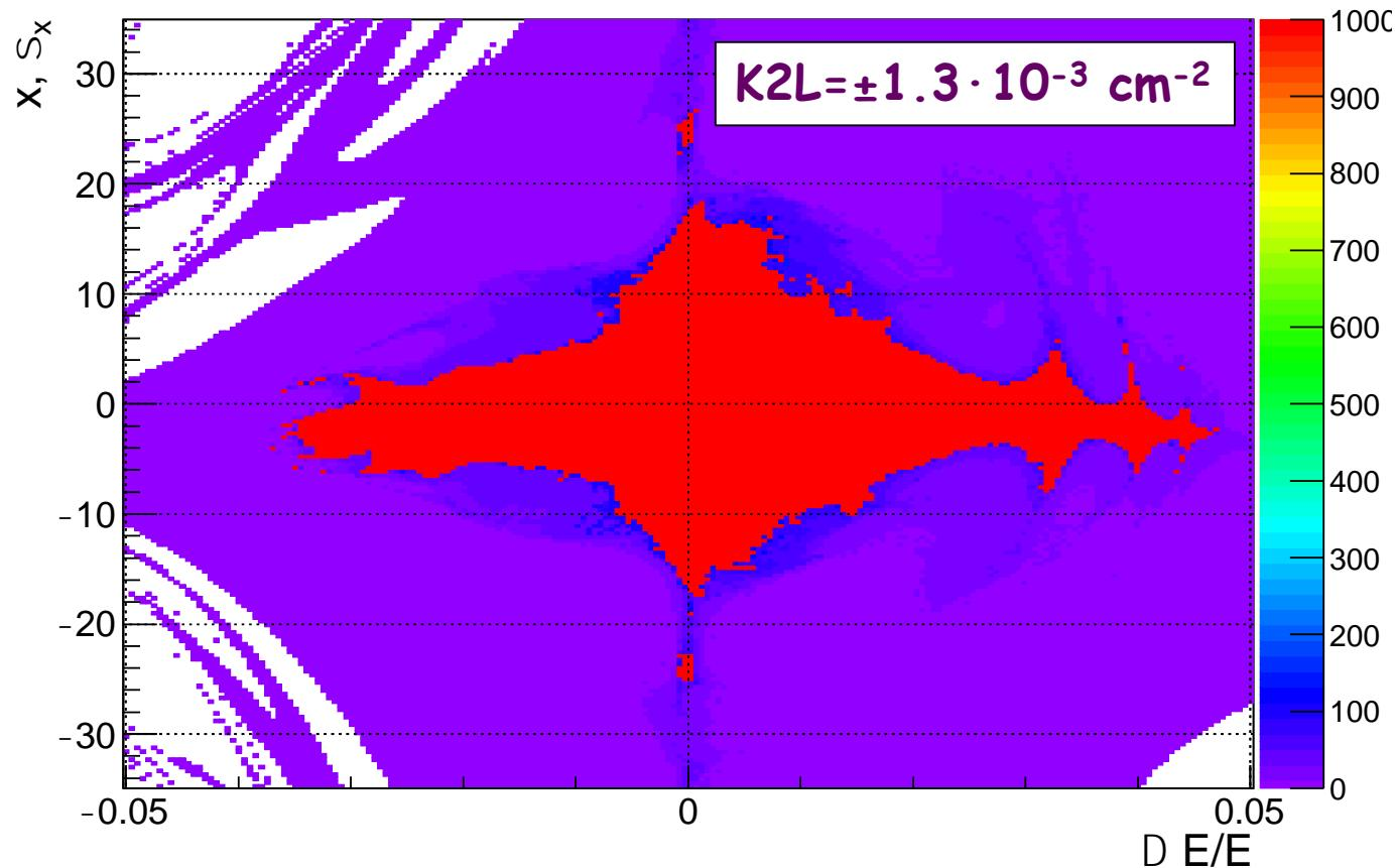
ε<sub>x</sub>=1.7 nm·rad, 0.2% coupling, σ<sub>x</sub>=1.6·10<sup>-3</sup>, |<sub>x</sub>~150 turns, Urf=2.5 GV
