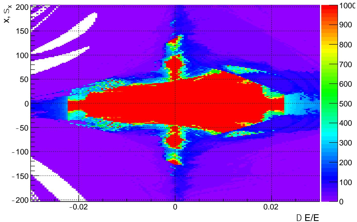
$\varepsilon_x = 0.11 \text{ nm} \cdot \text{rad}$ , 0.2% coupling,  $\sigma_x = 4 \cdot 10^{-4}$ ,  $|I_x| \sim 10^4$  turns,  $U_{rf} = 21 \text{ MV}$
