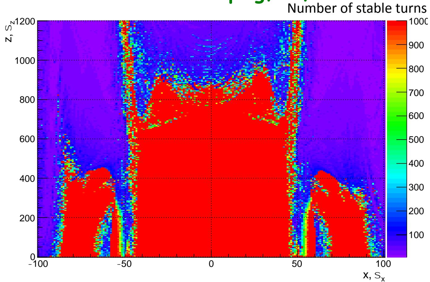
$\varepsilon_x = 0.11 \text{ nm} \cdot \text{rad}$ , 0.2% coupling,  $\sigma_x = 4 \cdot 10^{-4}$ ,  $|I_x| \sim 10^4$  turns,  $U_{rf} = 21 \text{ MV}$
