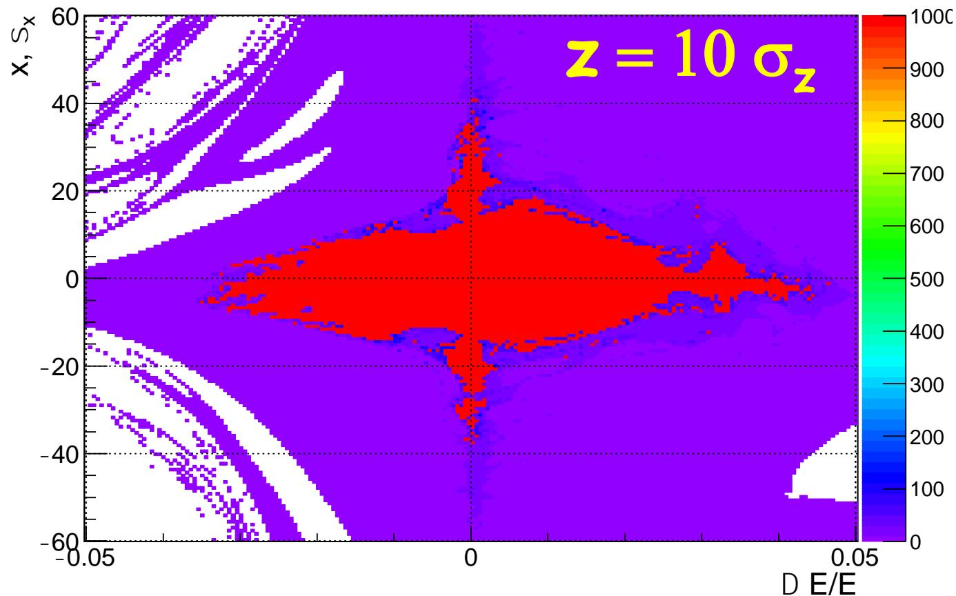
$\varepsilon_x = 1.7 \text{ nm} \cdot \text{rad}$ , 0.2% coupling,  $\sigma_x = 1.6 \cdot 10^{-3}$ ,  $|x| \sim 150 \text{ turns}$ ,  $U_{\text{rf}} = 2.5 \text{ GV}$
