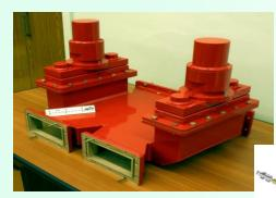
Adjustable directional couplers for TESLA (C = 3 ... 12 dB; adj. range  $\pm 1$ dB; D, R better than 30 dB.)
