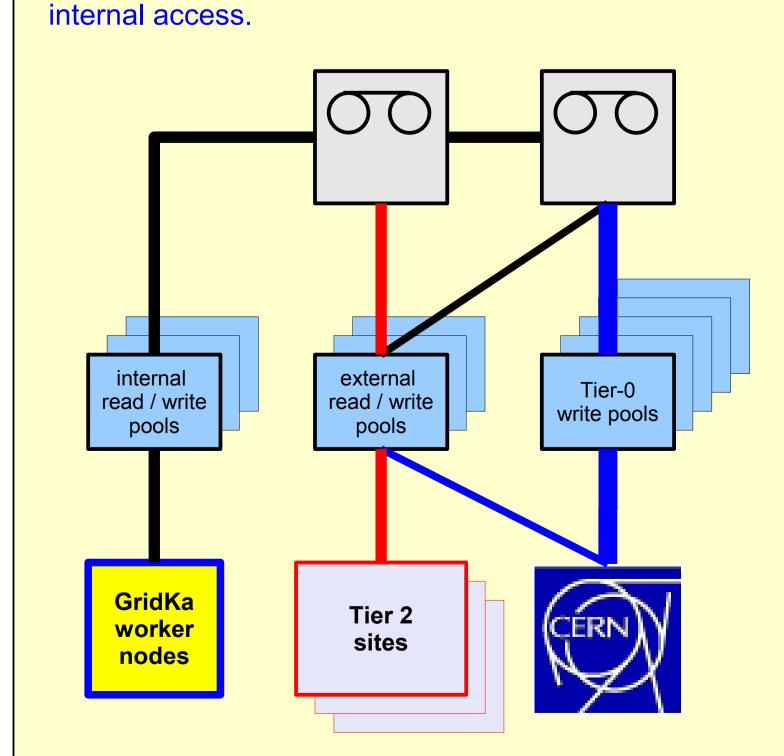
Picture shows a simplified view of the GridKa dCache setup.
