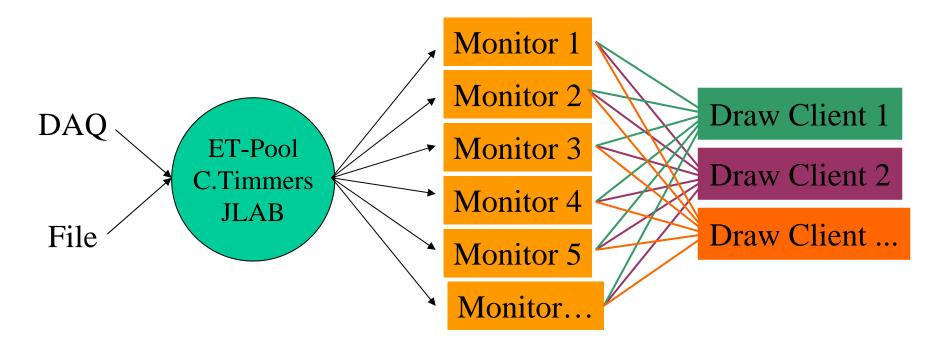
Simple client server architecture Information is passed via Root histograms Users only interact with the clients, no Pilot errors interfere with the monitoring The monitoring code has to survive millions of events
