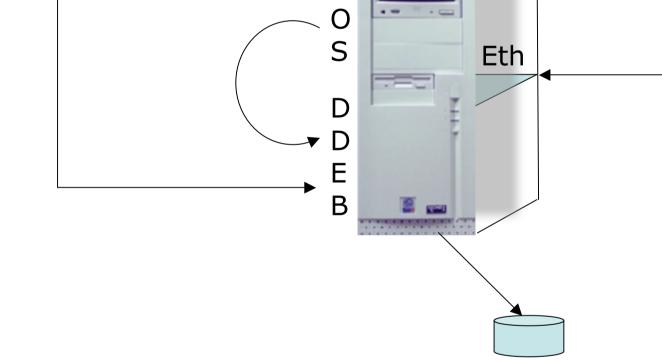
The MROD readout does not follow the standard ATLAS path (from the MROD to a ROS) via s-link), since we want to take detector commissioning decoupled from DAQ commissioning. Fragments are red out by the RCD via VME. Since data are already formatted as ROD fragments, RCD builds ROS fragments and sends them directly to the DDEB.
