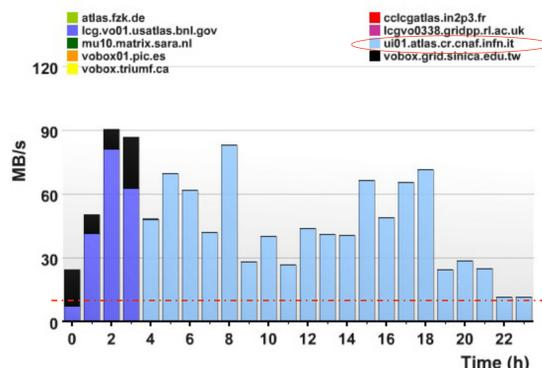
Preliminary test of data transfer between Tier 0 and Tier 1 (CNAF) during SC3. Without QoS, transfer rate is always above the required one.
