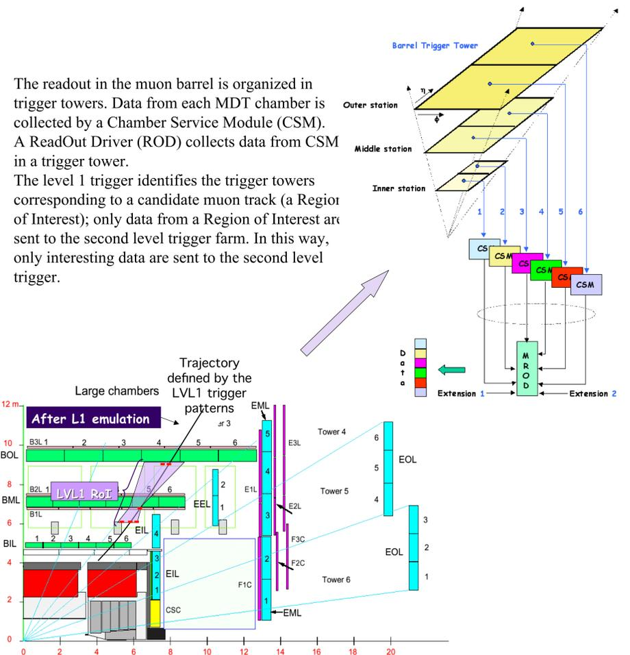
The readout in the muon barrel is organized in trigger towers. Data from each MDT chamber is collected by a Chamber Service Module (CSM). A ReadOut Driver (ROD) collects data from CSM in a trigger tower. The level 1 trigger identifies the trigger towers corresponding to a candidate muon track (a Region of Interest); only data from a Region of Interest are sent to the second level trigger farm. In this way, only interesting data are sent to the second level trigger.
