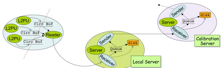
Software structure: the PU are separated from the reader by a buffer. Level 2 latency is only related to data preparation (O(200 μsec)).
