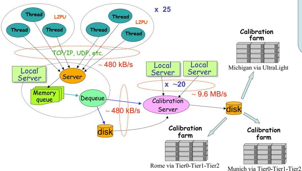
Data extraction procedure has been tested on the ATLAS preseries. Emulated L2PU produce data packets (1 kB/event) and send them to the local rack server. The local server packs data in 64 kB packets and sends them to a calibration server. The calibration server behaviour has been tested emulating 20 local servers sending data to it.
