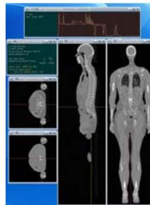
Fig. 1: A visualisation of the description of the body geometry in FLUKA obtained from an imported CT scan.
