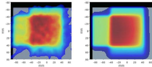
Fig.2: Comparison between a measured 3D map obtained from a post-irradiation PET scan and the FLUKA simulation.
