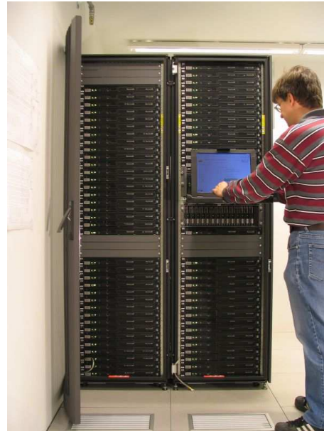
Figure 1: The 132 CPU Opteron cluster at the University of Helsinki is used for physics-, chemistry- and HEP-applications. The Ametisti cluster is part of the Finnish M-grid, which currently has 1118 AMD Opteron CPUs connected with the Advanced Resource Connector (ARC) middleware [10].
