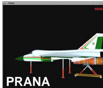
Iron bird – Hardware-in-loop simulator
