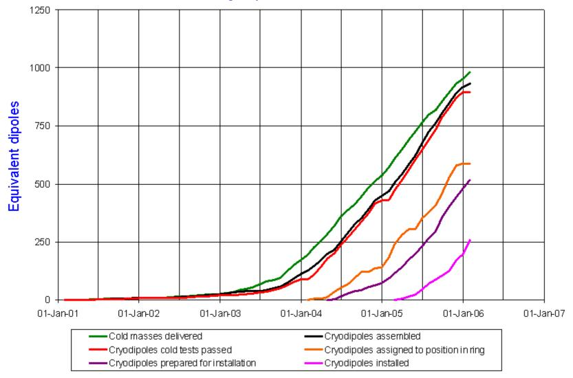
Data provided by D. Tommasini AT-MAS, L. Bottura AT-MTM
