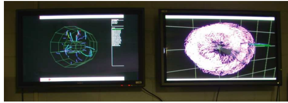
Figure 3: STAR Control Room plasma displays with near-real-time event displays, rendered with OpenGL.
