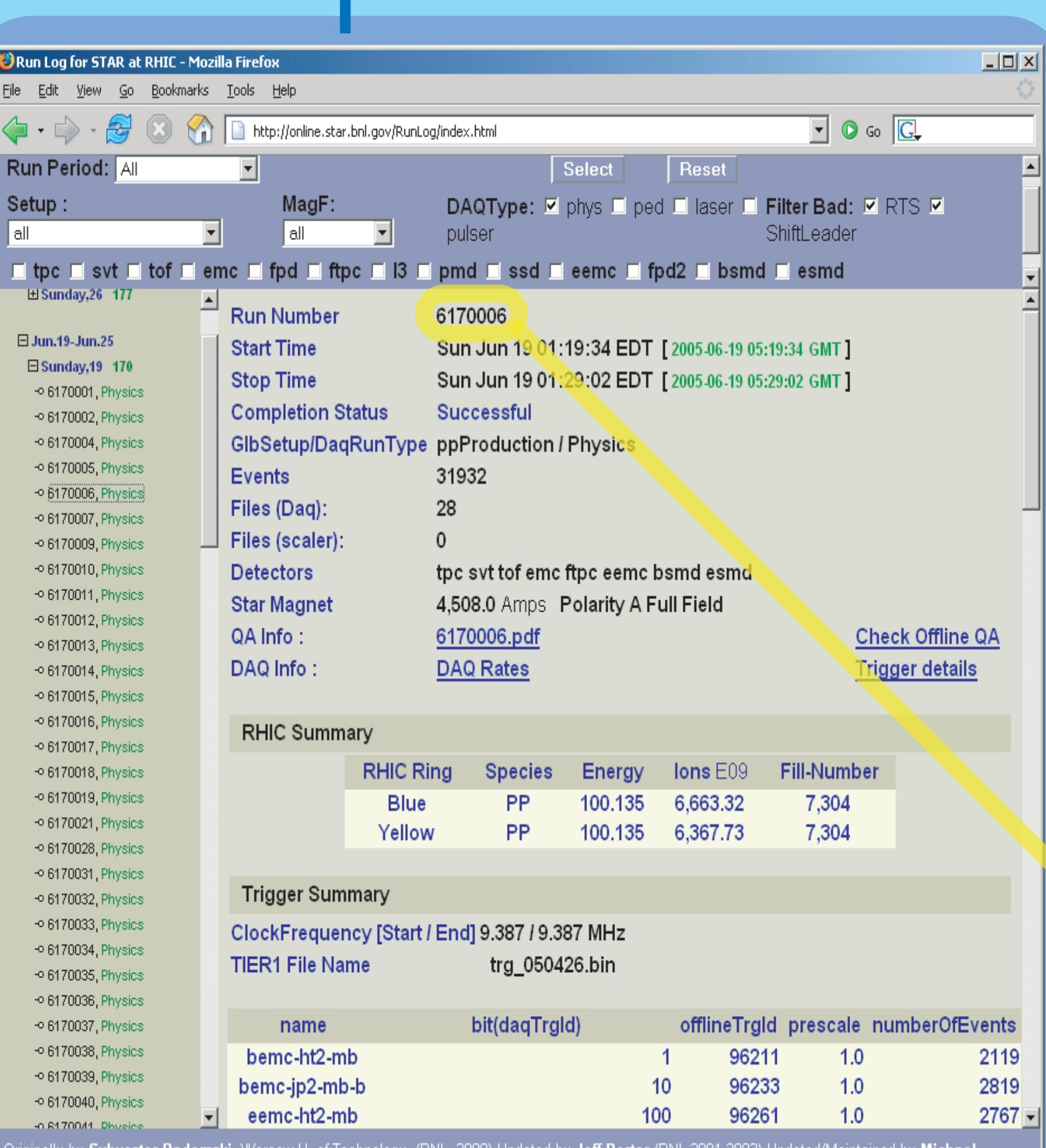
A frequently used tool to extract DAQ and run information is our PHP-based RunLog Browser. Essentially every detail about any particular run is available, such as detector states, number of events by trigger, collider status, and file storage, plus the software can create summary information covering multiple runs. Having helped collect this data, our collaborator's work has just begun, and he may return to these tools many times as he works to understand the experiment and the physics.
