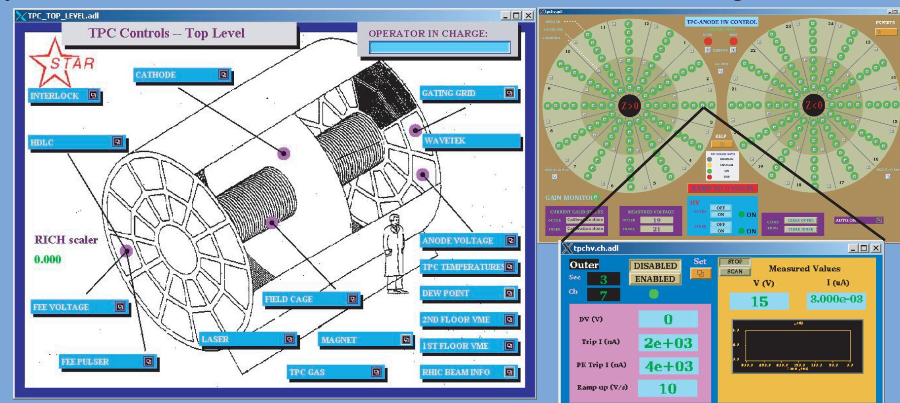
STAR Slow Controls consists primarily of EPICS-based readout and control of most subsystem parameters, though some subsystems rely on LabVIEW and various home-grown software. EPICS, hosted at Argonne National Laboratory, is a collaboratively developed set of Open Source software to create distributed soft real-time control systems.
