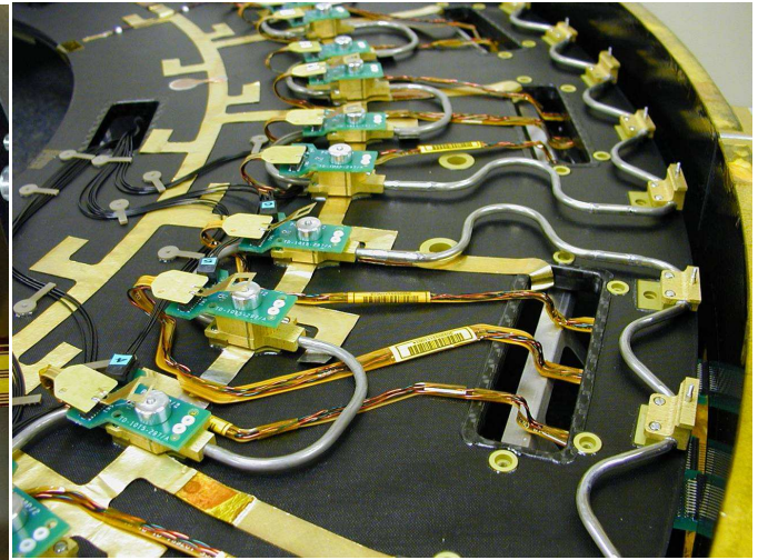
Figure 4 Photograph of section of a disk showing the power tapes, optical fibres and opto-package and the cooling pipes.
