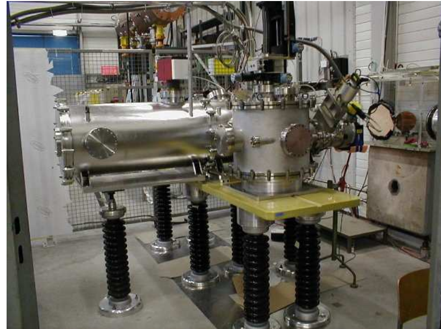
The prototype Laser Ion Source in building 236 on a HV platform ( \sim 100 kV) to decrease space charge
