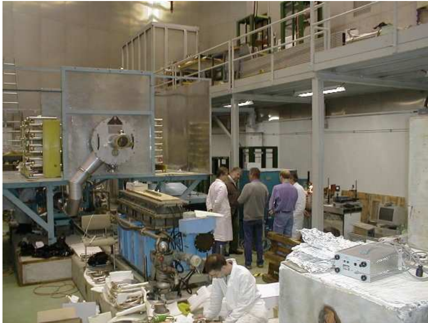
The Russian 100 J, 1 Hz CO 2 Laser Amplifier in building 363 (“Farady Cage”), being commissioned
