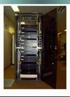
+Central Facilities (Non Grid) 250 CPUs 10TB Disk 35TB Tape (Capacity 330 TB)
