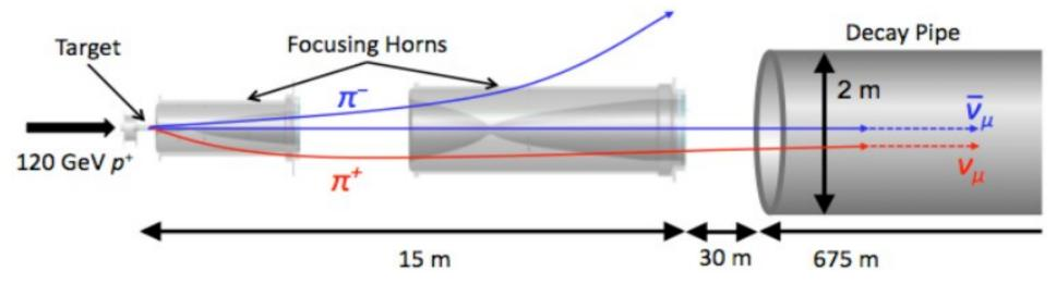
Neutrinos are created by in-flight decay of secondary/tertiary particles (mainly pion, kaon, and also muons)
