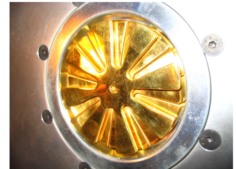
Failures of the Generating Voltmeter caused three Pelletron accesses
