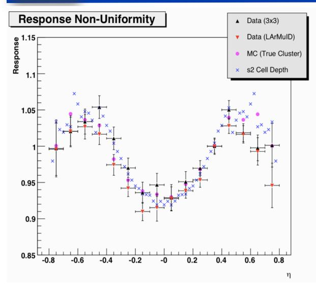
Three cluster MPV curves are shown - the LArMuID and 3x3 cluster algorithms applied to real cosmic data, and the true cluster from the cosmic simulation. The curves have been normalized to the point at eta between 0.3 and 0.4. Also shown is the second sampling cell depth. The MPV value clearly tracks the cell depth as one would expect for a minimum ionizing particle - the uniformity of the response agrees with simulation at the level of 2%.
