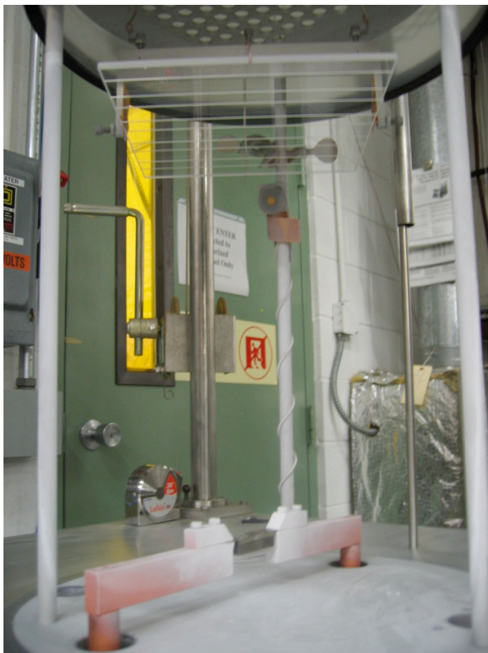
PTP evaporation setup, and quartz plate holder
