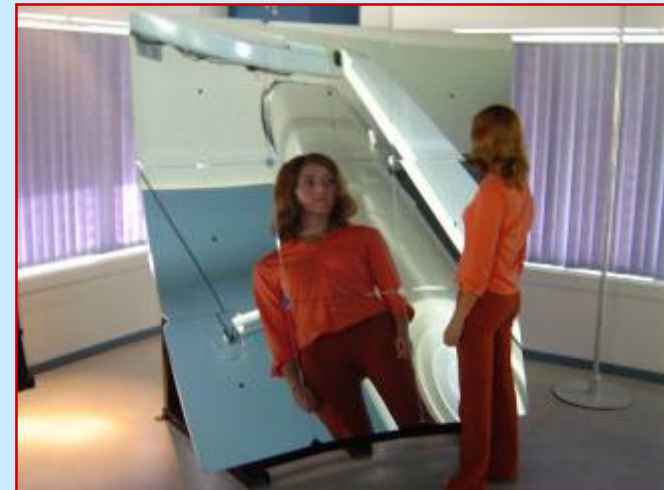
Quarter-size FD mirror set-up from Karlsruhe
