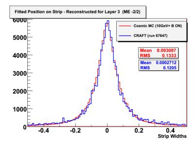
Cathode Strip Chamber response to cosmic ray muons are well described by a Monte Carlo simulation
