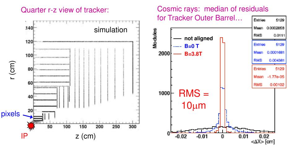
→ The quality of this cosmic ray alignment is comparable to what will be obtained with 10–50/pb of collision data
