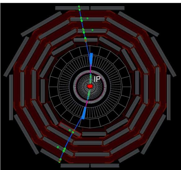
CMS Magnet: • 6m diameter • 13m long • 4T max field • Stored energy = 2.5GJ
