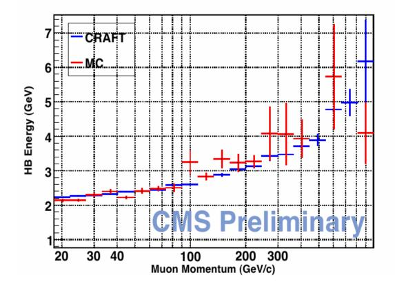
Hadronic calorimeter response to muons well described by a Monte Carlo simulation
