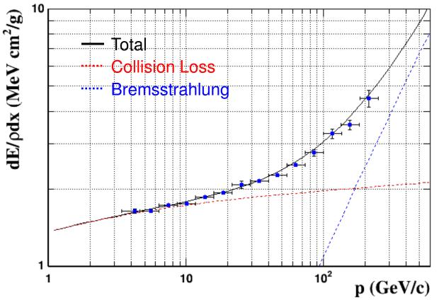
Energy loss per unit length for muons is well described by Particle Data Group's description of stopping power in PbWO<sub>4</sub>
