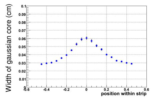
(Resolution is better at the edges of the strips because the charge is shared between strips)
