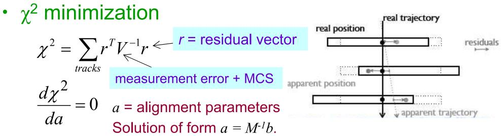
Requires matrix inversion: Full diagonalization (eg LAPACK) or fast solving techniques (eg MA27) - possible with sparse matrix.
