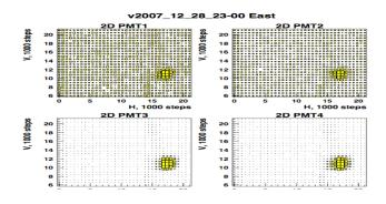
• Scanning is routinely done to reconfirm the centroid of the luminous spot.
