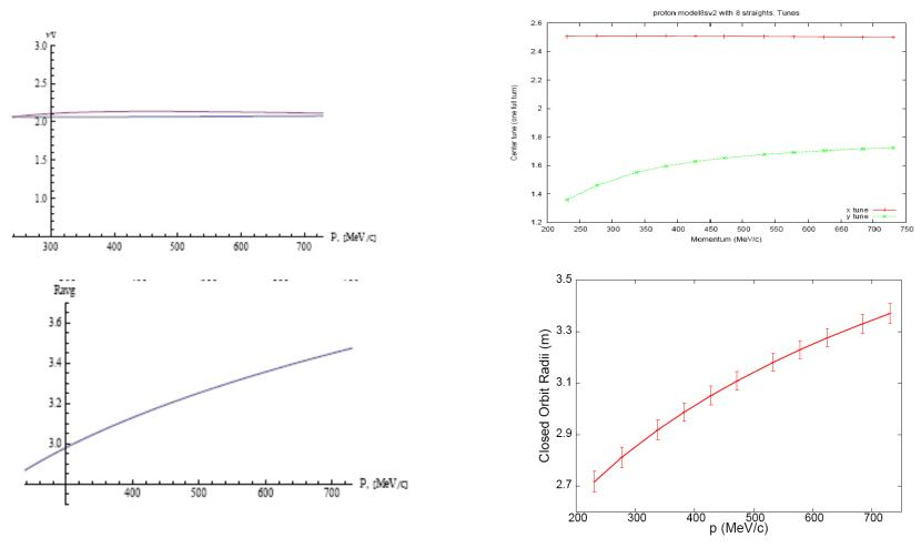
Large tune shift is due to the fringe field vs. the hard-edge model
