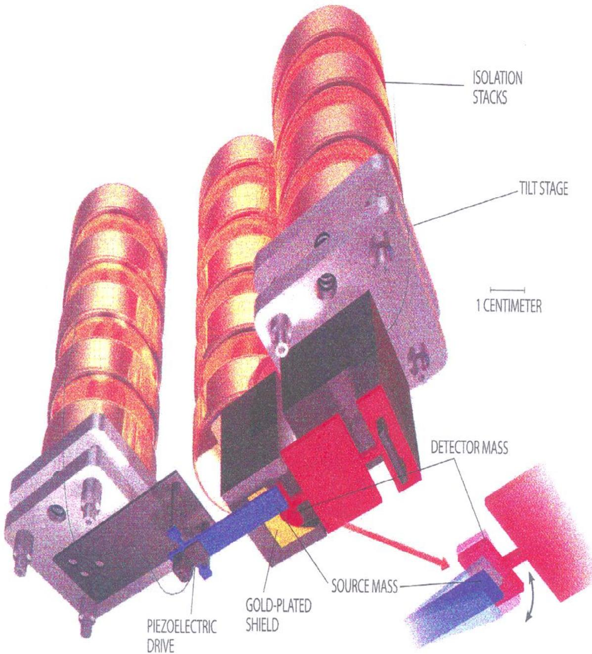
**TORSION OSCILLATOR** at the University of Colorado looks for changes in gravity from 0.05 to 1.0 millimeter. Piezoelectrics vibrate the tungsten source mass (blue) like a diving board. Any forces acting between the source mass and the tungsten detector (red) produce twisting oscillations of the detector (inset; oscillations are exaggerated), which are sensed by electronics. A gold-
