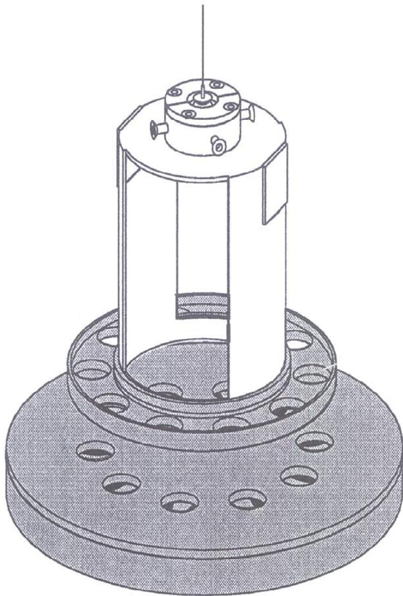
FIG. 1. Scale drawing of the torsion pendulum and rotating attractor. The active components are shaded. For clarity, we show an unrealistically large 1.5 cm vertical separation between pendulum and attractor, and omit the BeCu membrane and the attractor drive mechanism. The 4 horizontal screws were adjusted to make the pendulum precisely level.
