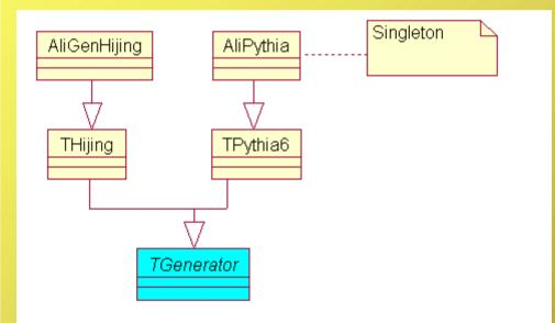
• Interface to external generators using the TGenerator class from ROOT
