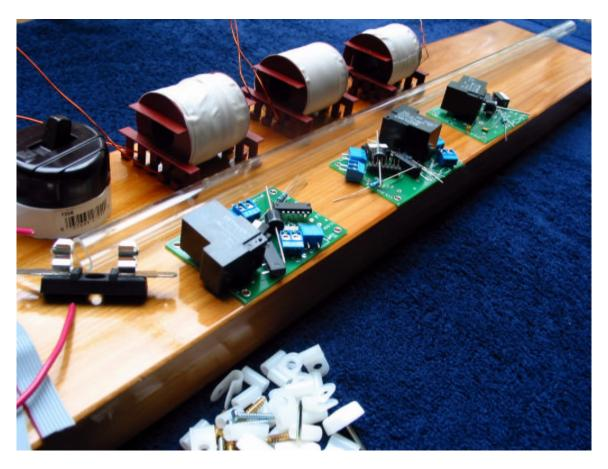
This is a picture of a pile of parts along with a 70cm long board that will, when constructed, turn into the next picture. It's estimated that construction can be completed in 8 to 10 man hours. Students will be required to solder components onto pc boards, wind a solenoid, and mount light sensors, drill holes and test electronic logic boards.
