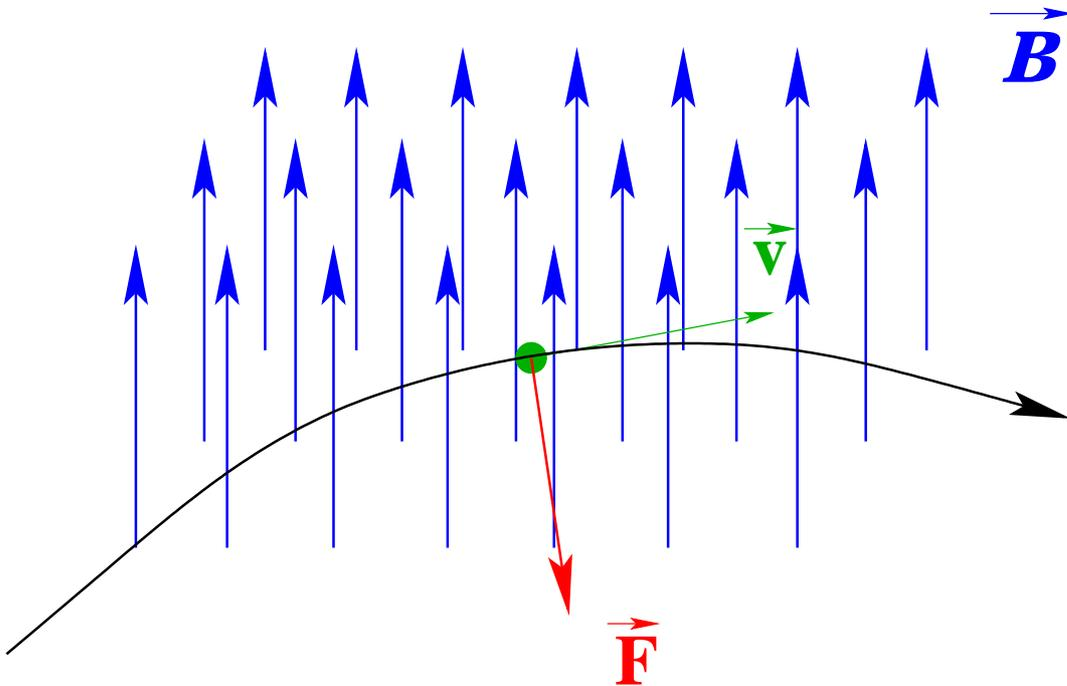
→ Trajectory curvature due to B field!
