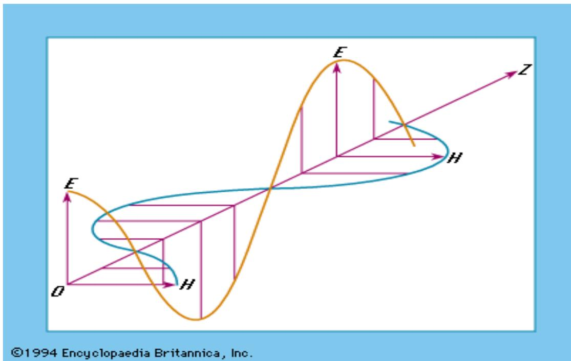
→ **No acceleration in the direction of propagation!**
