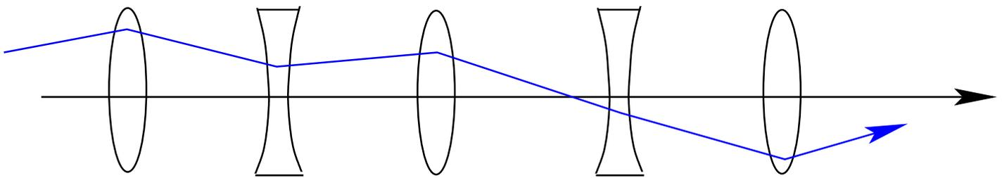
**Idea:** cut the arc sections in **focusing** and **defocusing** elements
