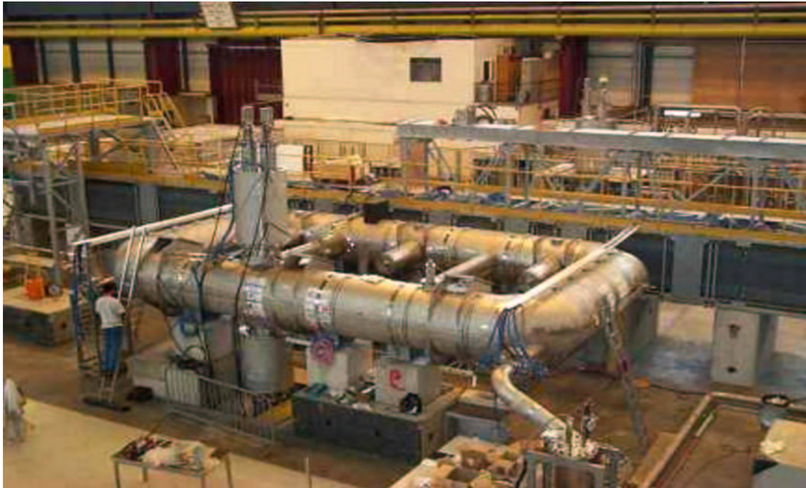
Each ATLAS BT coil will be separately tested in the surface hall
