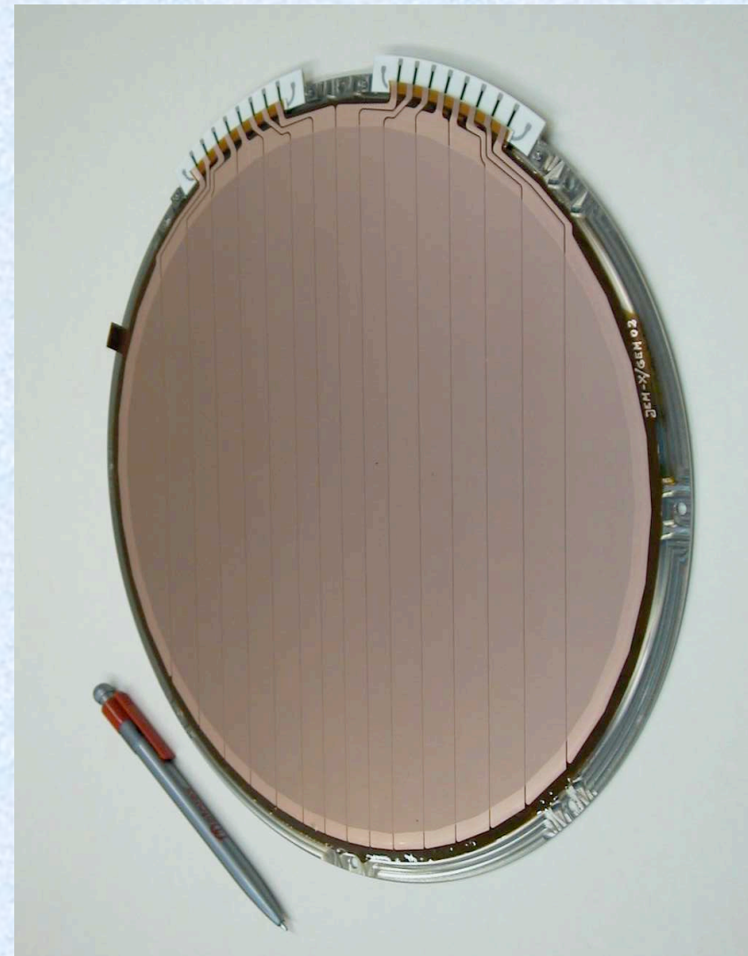
ESA-INTEGRAL Mission Prototype GEM for JEM-X (25 cm Ø):
