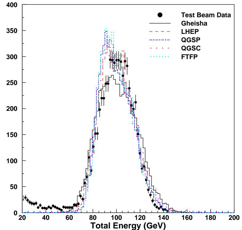
Worsening in resolution is due to non-matching e/h between ECal and HCal
