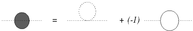
Figure 5. Radiative corrections to the mass of a scalar particle. The dotted curves are scalar propagators, and the solid curves are fermion propagators. (a) Diagrams with no supersymmetry, and (b) Diagrams with supersymmetry.
