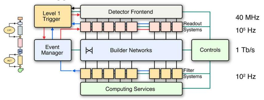
No. of In-Out units 512 Collision rate 40 MHz Level-1 Maximum trigger rate 100 kHz<sup>†</sup> ? 1 Terabit/s Readout network bandwidth Average event size ? 1 Mbyte ? 106 SI95‡ **Event filter computing power Event Flow Control** ? 10<sup>6</sup> Mssg/s Data production ? Tbyte/day No. of PC motherboards ? Thousands †50 kHz at startup (DAQ staging)  $\pm 6 \times 10^5$  at startup
