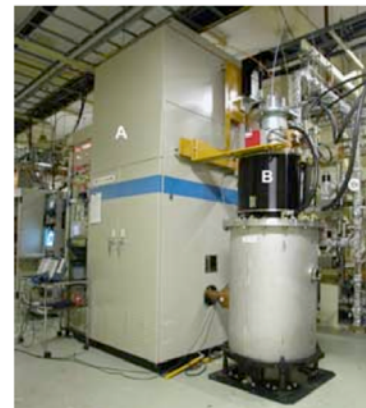
Fig. 2 : High power C-band (5712MHz) rf system. (A) Compact pulse modulator for klystron (350kV, 310A, 2msec, (flat top), 50Hz). (B) 50 MW high-power klystron (Toshiba E3748) assembly. (C) Waveguide to the C-band accelerator section.
