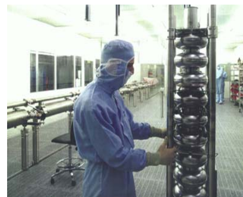
Cleanroom handling of niobium cavities
