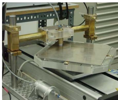
Eddy-current scanning system for niobium sheets
