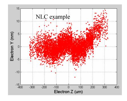
Disruption parameter is ratio of bunch length to focal length:  $D_y = \frac{\sigma_z}{f_y} = \frac{2r_e N \sigma_z}{\gamma \sigma_x (\sigma_x + \sigma_y)}$
