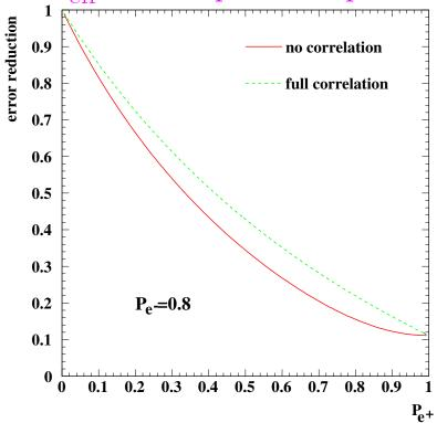
With  $\mathcal{P}_{e^+} = 60\%$  a factor 3-4 is gained in the precision of  $\mathcal{P}_{\text{eff}}$
