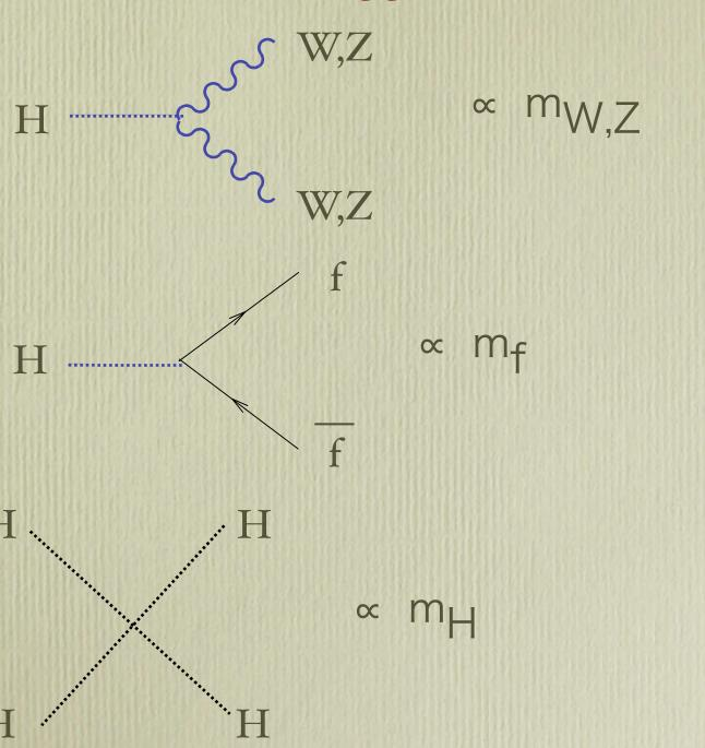
More complex interactions can be built out of these building blocks, by enforcing the laws of conservation of energy, momentum, and charge. The calculational rules associated to each vertex and to the propagation of the intermediate states (the lines connecting different vertices) allow to calculate in a unique way all the properties of more complex interactions.
