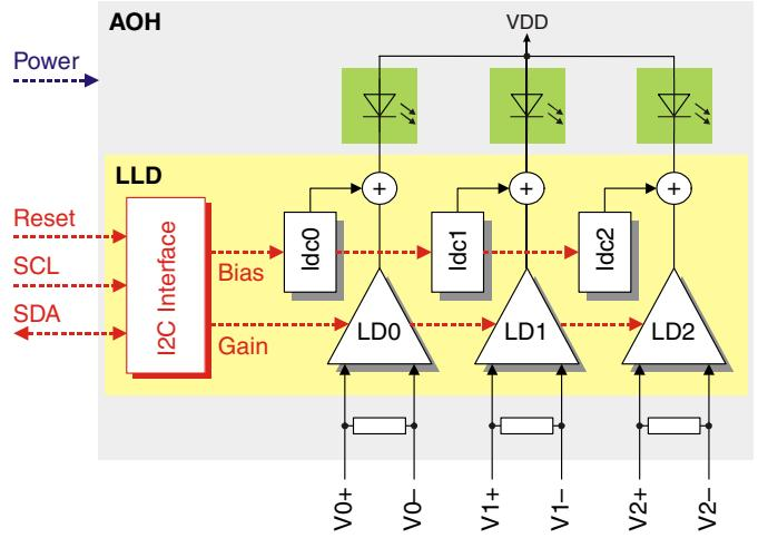
Figure 4: Block diagram of the Analog Optohybrid (AOH) and the Linear Laser Driver (LLD) ASIC contained within.
