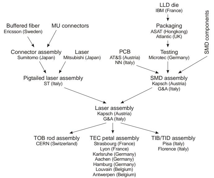
Figure 5: Flow of components around the SMD and laser assembly of the Analog Optohybrid (AOH) manufacturing.
