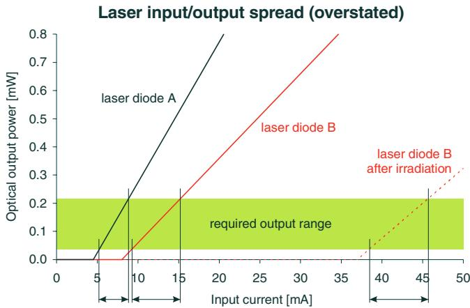
Figure 3: Exaggerated sample spread of the input/output characteristics of the laser diodes. The shaded area indicates the optimum light output power range, which can be reached by individual bias and gain settings in the Linear Laser Driver (LLD).
